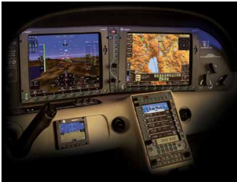
L-3 Avionics Systems' SmartDeck with synthetic vision and its Trilogy ESI-1000 electronic standby instrument.
